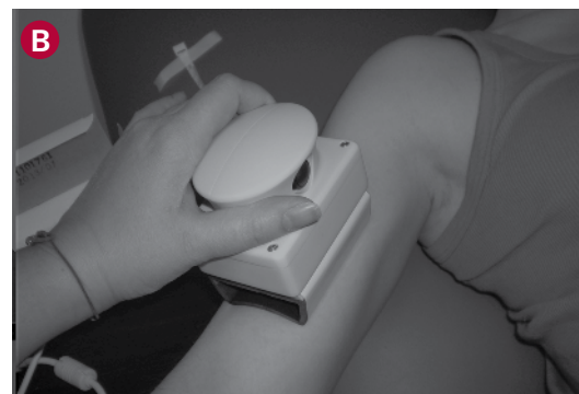
Figure 1. Electrical impedance myography. (A) A portable device with a simple hand-held wand is used to measure impedance over selected muscles. (B) Each measurement takes seconds.
